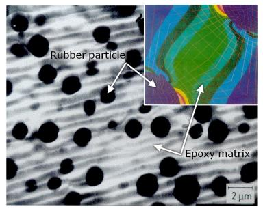
**Rubber toughened epoxy adhesives:** when the material is stressed (e.g. at a crack tip), there will be triaxial tensile stresses acting on the rubber particle due to the different elastic moduli and Poisson ratios of the rubber particle and the matrix. This leads to cavitation of the rubber particles which enables plastic void growth, and hence a large increase in the toughness. Inset: the stress field.
