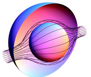
**Metamaterials:** it has recently been noticed that the optical properties of a material may be tailored by adjusting its microstructure as well as its chemistry. Simulation has been used to design such metamaterials, which can even be made to have a negative refractive index. Applications include a perfect lens and an electromagnetic cloak, depicted
