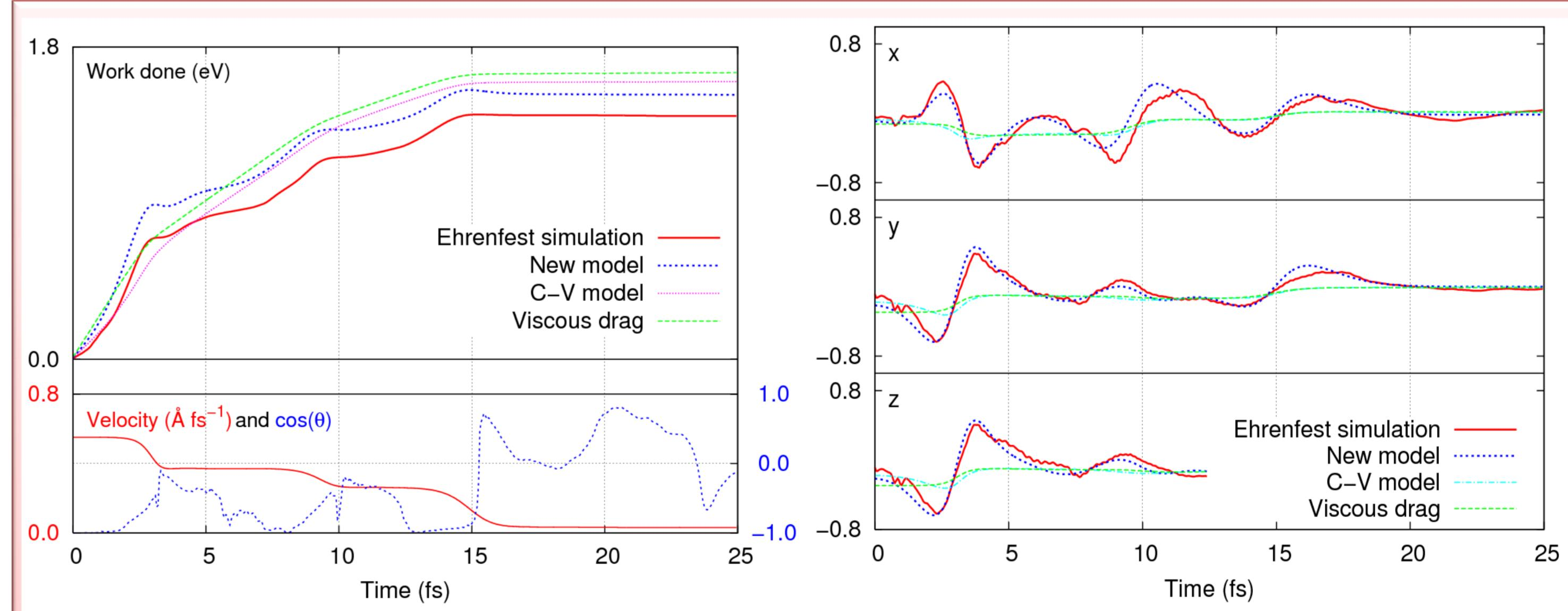
Our model reproduces in detail the non-adiabatic forces on individual atoms during a collision and so captures the work done by non-adiabatic forces with unprecedented accuracy. (Left): the upper panel shows the work done by  $F_1$  acting on a PKA in a sample Ehrenfest simulation of a collision cascade. The lower panel shows  $\mathbf{v}$  and  $\tilde{\mathbf{v}} \cdot \tilde{\mathbf{F}}_1$ . (Right): the Cartesian components of the non-adiabatic force (in eV/A).
