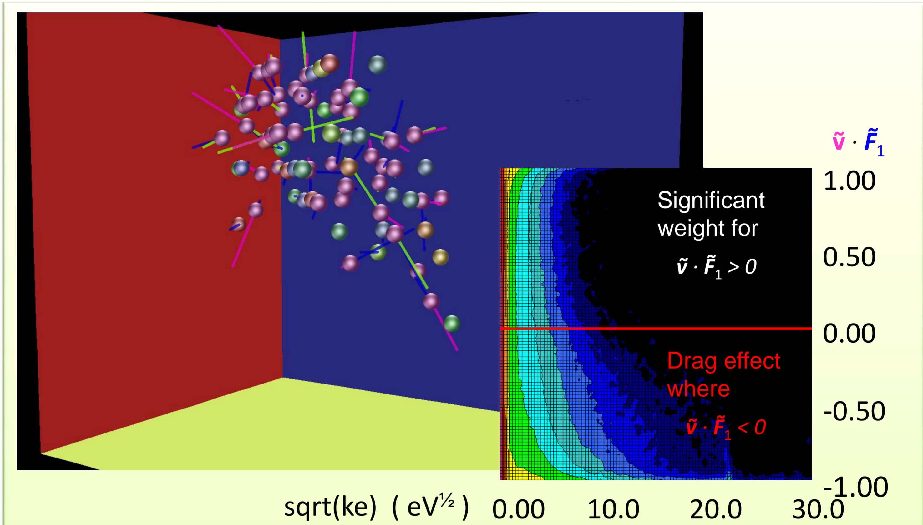
30fs into a 1keV cascade in 2016 atoms computed quantum mechanically within the Ehrenfest approximation. **Velocity  $v$** , **Hellmann-Feynman force  $F$** , and **non-adiabatic force  $F_1$**  vectors shown.  $F_1$  is scaled for clarity. Note  $F_1$  is neither antiparallel to or proportional in magnitude to  $v$ . Inset: histogram of the cosine of the angle between unit vectors  $\tilde{v}$  and  $\tilde{F}_1$ .
