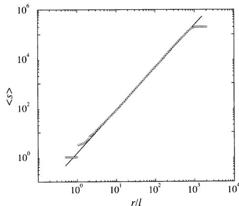
**Figure 2.** Log-log plot of average mass  $S(r)$  within distance  $r$  to a given particle as a function of  $r$  for two-dimensional, off-lattice DLA. Filled circles are experimental data, obtained from the DLA cluster shown in figure 1 as explained in the text. The line corresponds to the fit  $S(r/l) = 1.5 (r/l)^{1.74}$ , indicating a fractal dimensionality of  $D_f = 1.74$  of the cluster.
