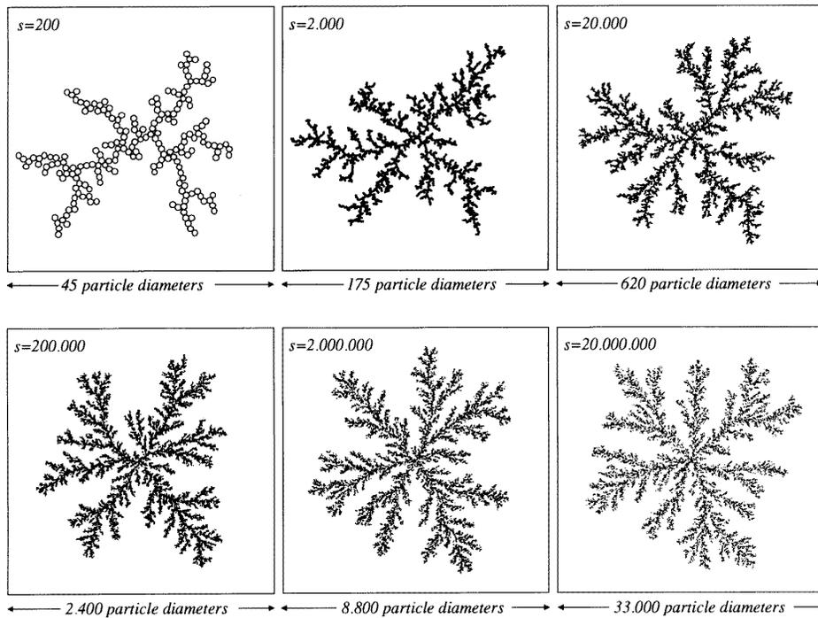
**Figure 1.** A two-dimensional, off-lattice DLA cluster at six different stages of growth. The cluster consists of identical discs of diameter  $l$ , and is shown at the stage when it contains  $s = 200, 2000, 20\,000, 200\,000, 2\,000\,000$  and  $s = 20\,000\,000$  particles respectively. The cluster seed was one single disc. According to the finite printer resolution, only a fraction of all particles are shown for  $s > 20\,000$  in order not to change the visual appearance of the cluster.
