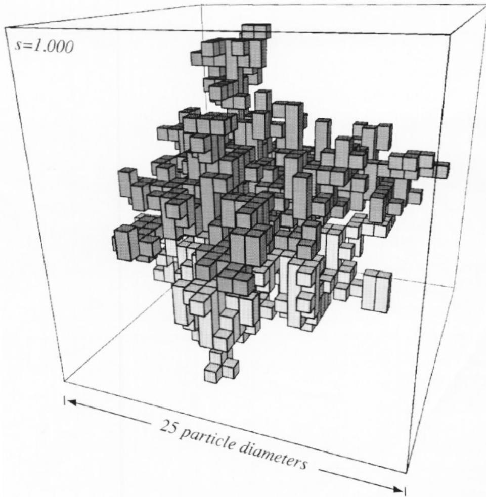
**Figure 3.** Perspective view of a three-dimensional, cubic lattice DLA cluster of mass  $s = 1000$ . The individual particles are identical cubes of side length  $l$ , but the cluster is displayed as if consisting of vertical columns of different lengths. The 'upper' and the 'lower' part are indicated (compare with the text).
