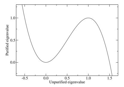
**Fig. 3** The purification transformation illustrated in terms of its effect on the density-matrix eigenvalues (occupation numbers).
