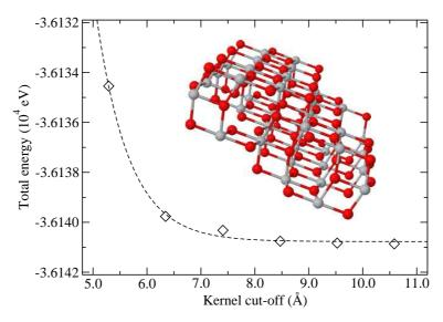
Fig. 4 Total energy convergence with respect to density-kernel cut-off  $r_K$  for a  $Ti_{38}O_{76}$  cluster [46].
