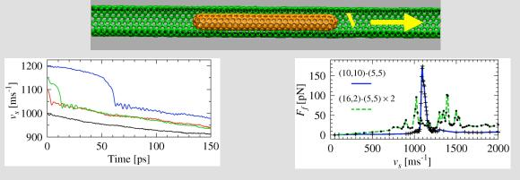
Molecular dynamics simulations of carbon nanotubes sliding relative to one another reveal a dramatic slowdown within narrow velocity ranges. This effect depends strongly on the atomic level structures of the tubes.
