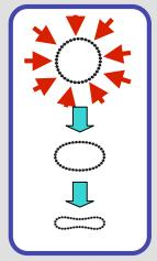
All single-walled carbon nanotubes deform under pressure, but how they deform depends on their diameters. Small nanotubes gradually change their shapes whereas larger tubes abruptly collapse.
